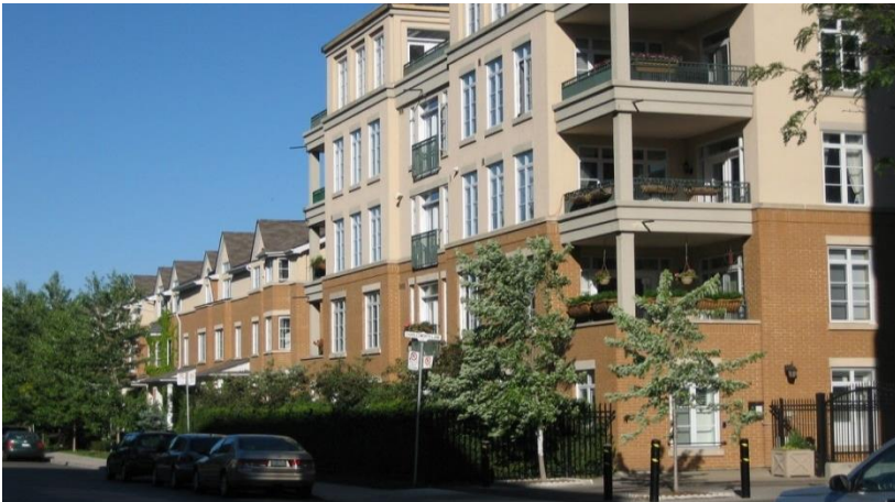
Photo 22: Building articulation and colour variation that helps create a gradual transition from one density to another should be considered to achieve a visually comfortable pedestrian scale.
