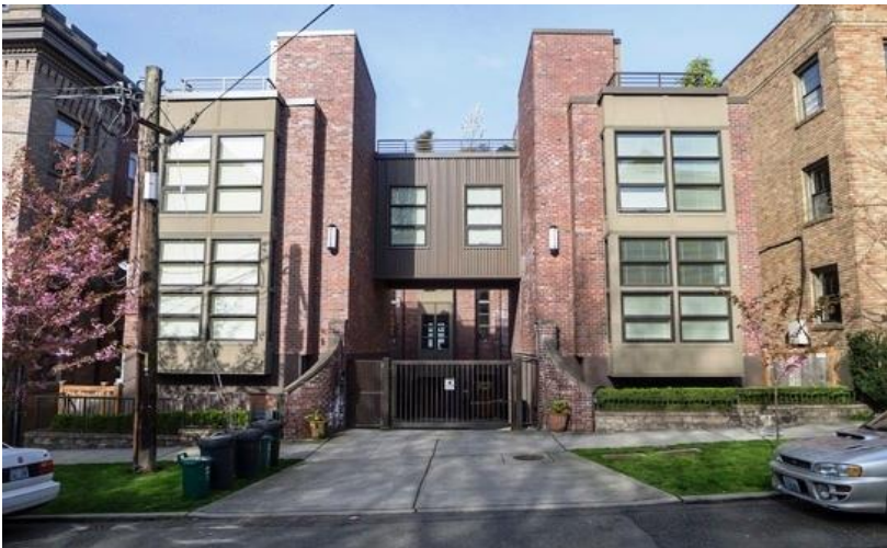
Photo 23: Building entrances can be highlighted through the use of canopies (above) or recessing the entrance wall from the primary face of the building (below).
