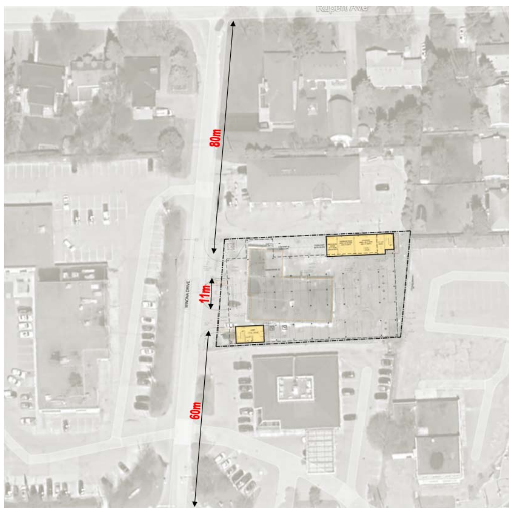
Figure 14 - Site Access Spacing via Google Maps
