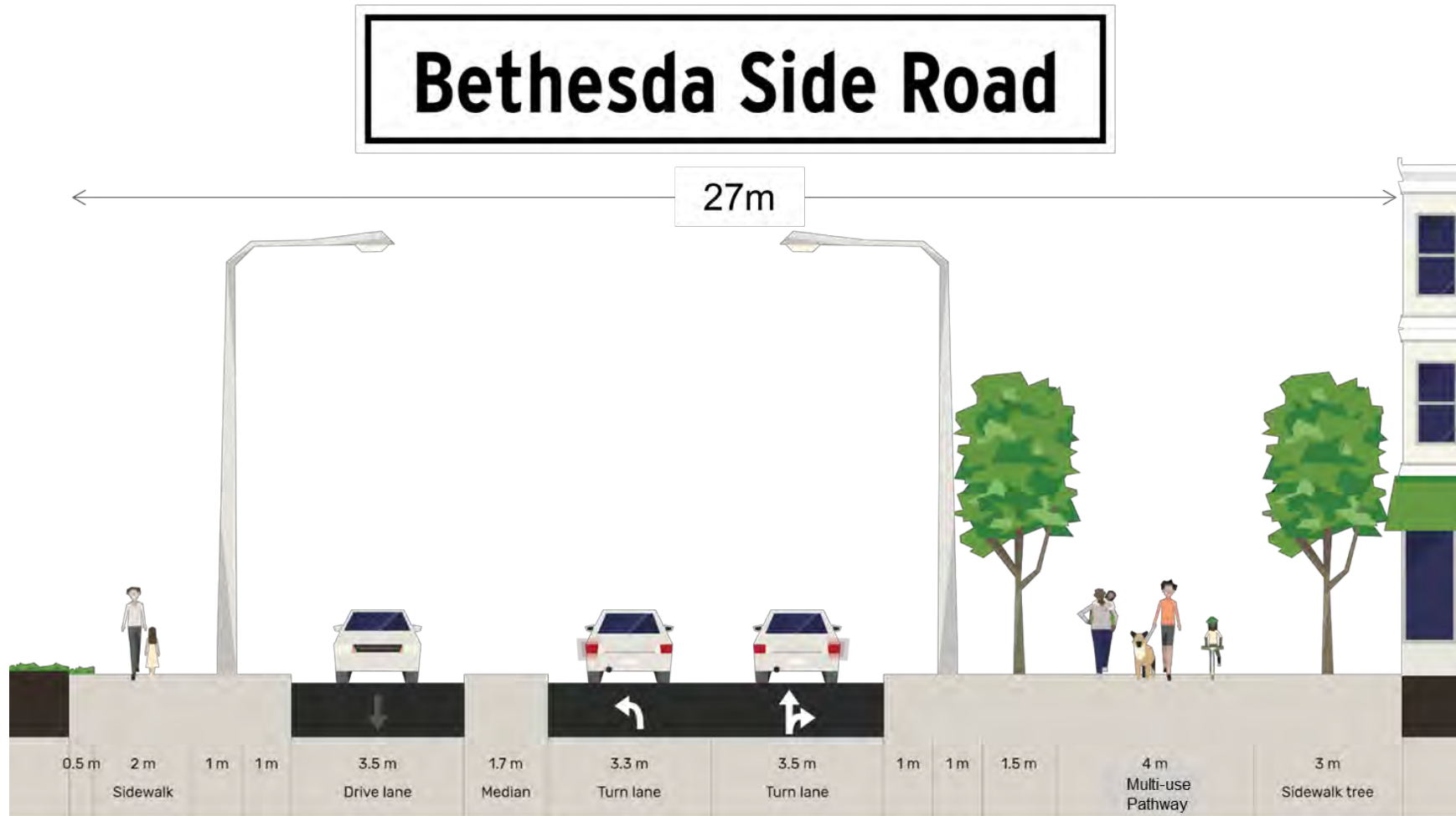
Exhibit 25: Conceptual Typical Cross Section for Bethesda Side Road, Intersection Approach with Left-Turn Lane.
